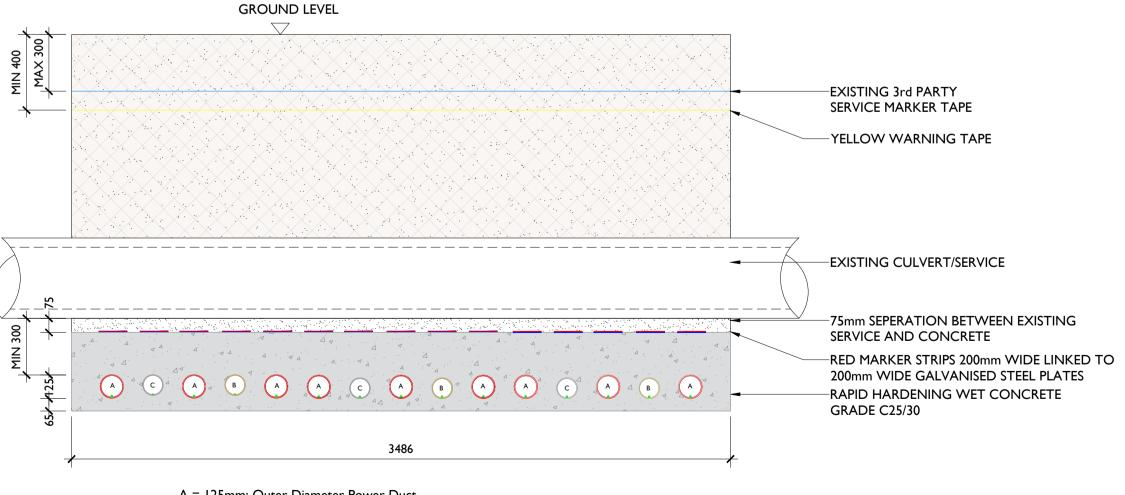
A = 125mm: Outer Diameter Power Duct, B = 110mm: Outer Diameter Comms Duct, C = I I0mm: Outer Diameter ECC Duct
